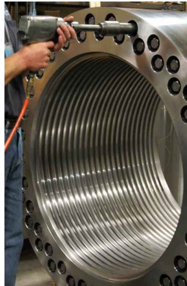
Assembling an enormous 1016 mm (40 inch) thread tensioner, used on a 50,000 ton press.
